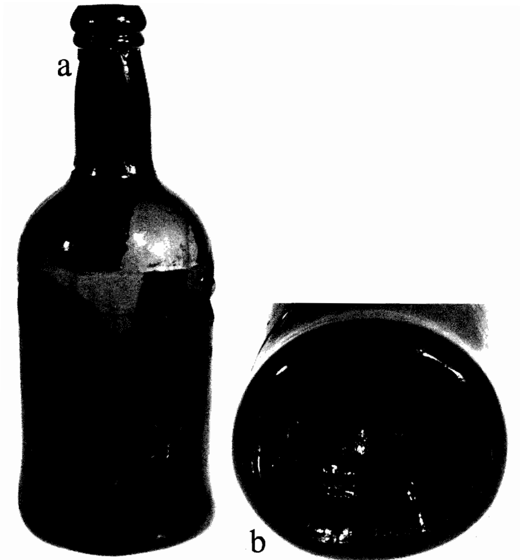
Figure 64. Blown in a three-piece mould, this bottle has a distinctive finish shaped by a finish-forming tool, a distinct basal sag, and a mould line on the heel (b). Based on the latter two features the bottle dates to the 1820s or early 1830s. (Photos by R. Chan; RA-12737B; RA-12733B)
