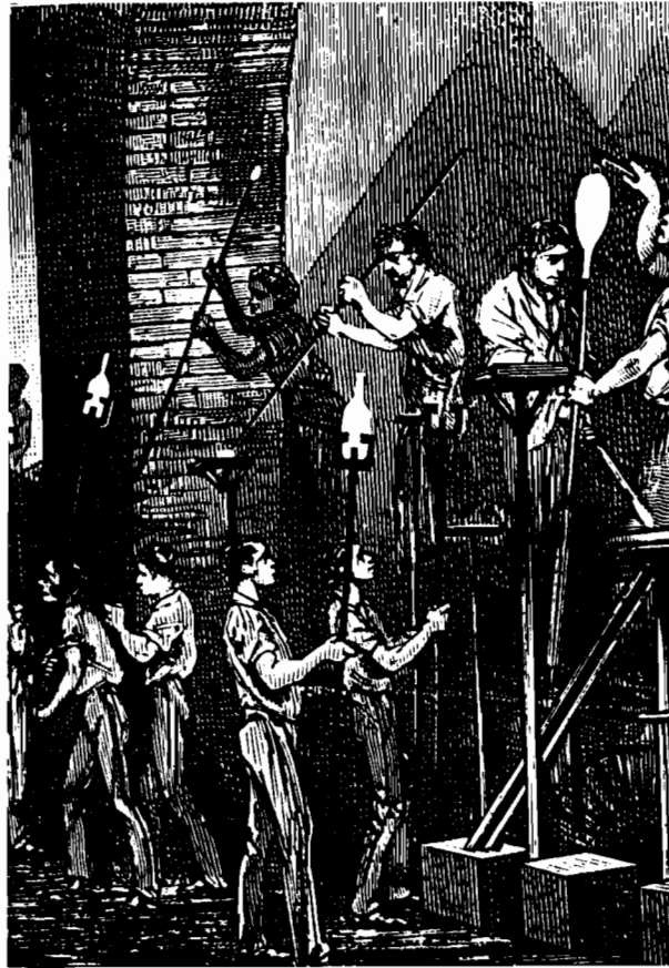
Figure 71. The snap or sabot , introduced sometime in the 1840s, replaced the pontil and left no mark on the base of the bottle. (Peligot 1877: Fig. 47. Photo by G. Lupien; RD-245M)
