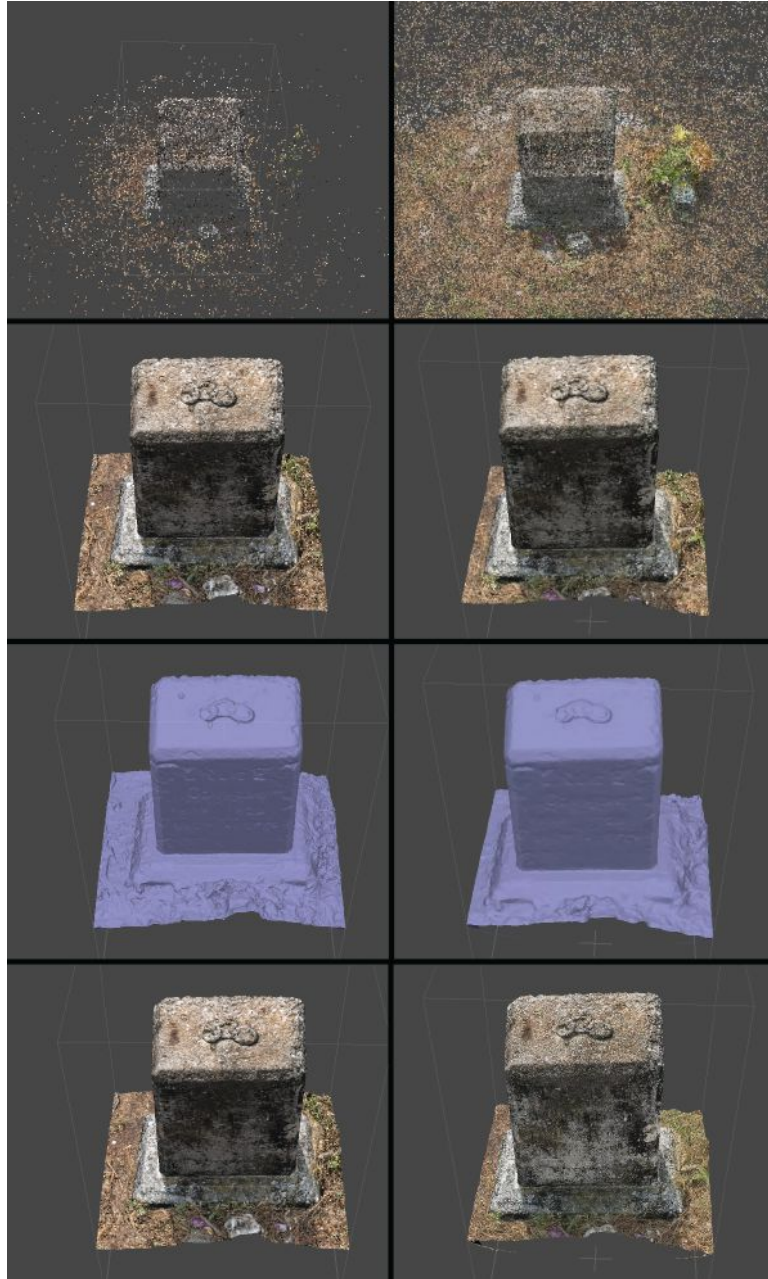
FIGURE 1. This illustration shows the differences (in the right column) that result from neglecting the Reconstruction uncertainty, Reproject error, Projection accuracy, and Optimize Cameras settings for the Lillie Conyers grave marker.
