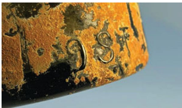
FIGURE 7. A typical scar on a semiautomatic machine-made bottle.
