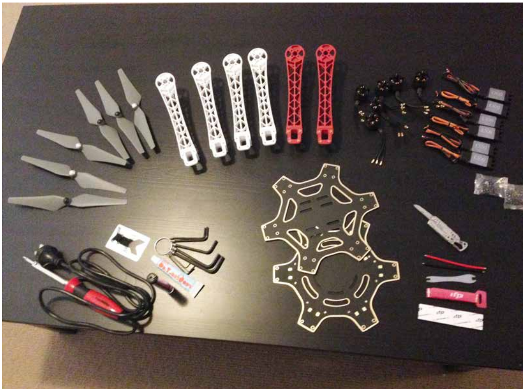
Figure 3. DJI F550 kit and tools used for assembly. (Photo by author, 2014.)
