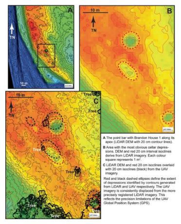
FIGURE 8. Comparison of the UAV and LiDAR elevation models for portions of Brandon House 1.
