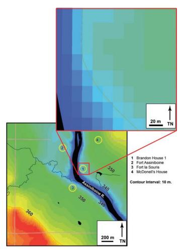
FIGURE 3. GIS rendering of the NTS shapefiles and 15 m resolution elevation model. The point bar terrace upon which Brandon House 1 is located is not detected.
