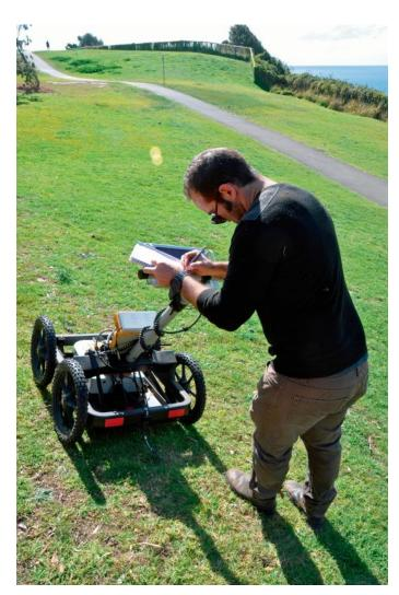
FIGURE 2. GPR in action to find the entrance of the World War Two observatory position. (Photo courtesy of O. Rochecouste, Macquarie University.)
