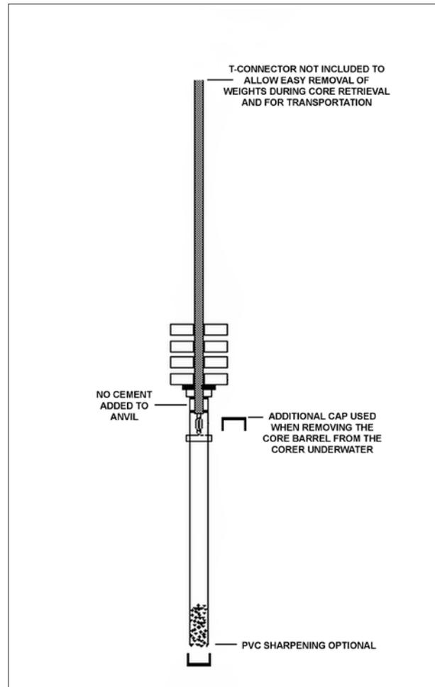
**Figure 2.** The author’s modifications to the coring device are simple, and yet allow the device to be more versatile and effective in the marine environment. (Drawing by author, 2007.)
