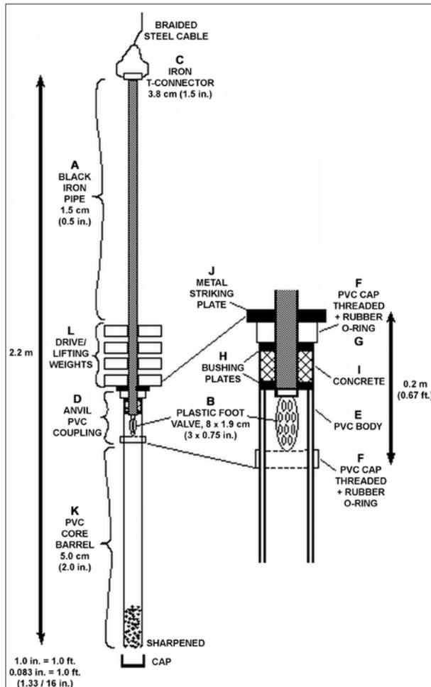
**Figure 1.** Cawley and Parker’s 2001 design for a diver-assisted percussion coring device, after Cawley and Parker (2001). (Drawing by author, 2007.)
