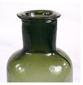
(*Figure 9 [above right].* A flared finish on an ink or utility bottle produced by an eastern American glasshouse ca. 1840-1860.)
