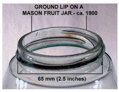
differently shaped bottle with a wider mouth or bore. The rough cracked-off top surface of this finish was subsequently ground off to make it uniform and flat, i.e., a ground rim. In general, with the exception of simple straight finishes (simply sheared or cracked-off upper neck ends which were mold-formed) and canning jars, bottle molds with incorporated finishes (in whole or in part) were little used until the late 1870s, receiving only limited use until the 1890s when they
