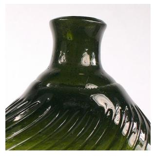
As with the previous two methods, shearing was both a blowpipe removal method and a type of simple finish. It entailed detaching the blowpipe from the bottle with some type of shears similar to tin snips or sheep shears—that cut the hot glass analogous to cutting thick plastic with scissors (Barber 1900:21). The resulting finish – which usually received some simple tool work to smooth out the edge - is called a Sheared Lip or Sheared Finish (**Fig. 4**).
