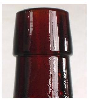
(*Figure 18 [to right above].* A tooled single-part finish, such as would be produced by the tool in Fig. 17. Note the horizontal striations on the finish and upper neck.)
