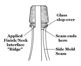
**the bore, if it will fit.** (**Fig. 16**) This line or ridge marks the interface between the blowpipe severing point and the separately applied finish glass; it can vary from obvious to non-existent (Boow 1991:64).
