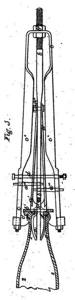
glass which was then shaped with a specialized tool (Hemingray 1860; Howard 1950; Jones 1986). Specifically, a variably thick (depending on the finish type and size desired) strip of hot glass was added at the blowpipe removal point using a pontil rod or other tool ("ring iron"). This was done as the bottle was rotated by another glassworker holding it by the base using either a pontil rod or a snap ("snap-case") tool (McKearin and Wilson 1978:13-14; Jones and Sullivan 1989:21).
