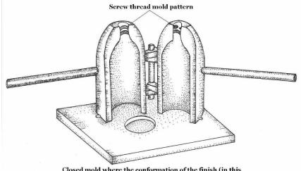
Closed mold where the conformation of the finish (in this case external screw threads) are formed by the mold itself.
