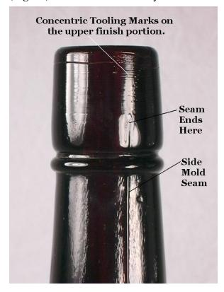
mold, the finish shape and bore conformation was made more precise—to ensure proper closure fit—with minor re-firing and/or tooling of the extreme upper portion of the finish (Deiss 1981).
