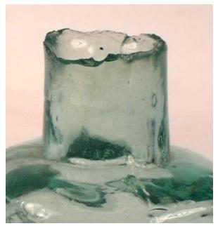
These are described in Lindsey [2009]. The same source includes a period film clip [very early 1900s] of a mouthblown "shop" blowing bottles using the burst-off method to detach the blowpipe.)
