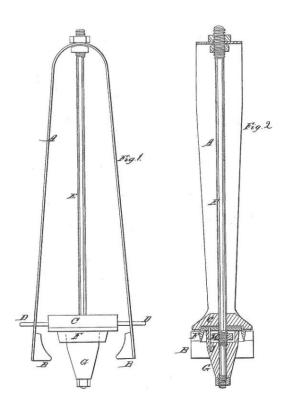
then...[formed with]...the plastic glass by a tool adapted to the purpose. This process is necessarily slow and laborious and the work when completed is not so uniform and complete as when the jar is finished in the mold and at one operation...[the latter of which was the purpose of the specific patent] (Hemingray 1860).
