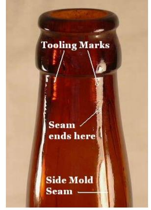
**2.** Concentric horizontal tooling marks are usually present on both the finish and the upper portion of the neck above where the side mold seam fades or disappears (Fig. 27).
