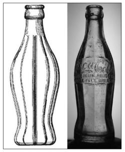
Figure 4 – Comparison of 1916 patent drawing with actual bottle
