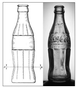
Figure 22 – Comparison of 1923 patent drawing with actual bottle
