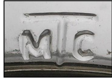
Figure 20 – MTC mark on Heel
