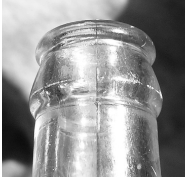
Figure 2-26 – Close-up of Side Seam and Finish – Machine-Made Bottle
