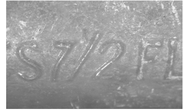
Figure 2-28 – Closeup of ½ Engraver’s Error
