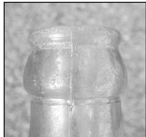
Figure 3-28 – Typical machine finish – Silver City Beer & Ice Co. bottle
