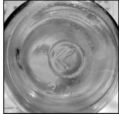
Figure 5 – L in ejection scar (eBay)
