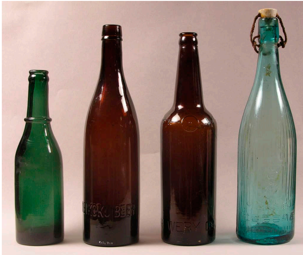
Figure 1. Japanese beverage bottles from North American sites (left to right): Mitsuya Cider (turn mold, height 23.8 cm); Teikoku Beer (three-piece mold, height 29.9 cm); Dai Nippon Beer (Owens machine, height 28.7 cm); Hakutsuru Sake (three-piece mold, height 30.6 cm). (Photo by author, 2008.)
