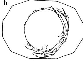
Figure 22. An Owens suction scar caused by shearing the glass when the mould is full (see Fig. 16b). The shears cause the glass surface to cool slightly, leaving a scar from the cutting action. (a) Also shows the base and heel mould seams from the parison mould.
