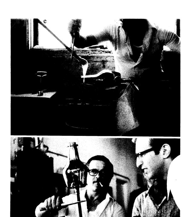
Figure 1e, 1f. (e) Hot glass is added to the neck to form the string rim. (f) A completed bottle.
