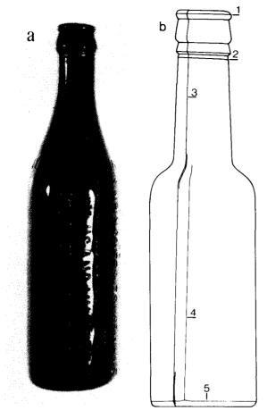
Figure 19. Two bottles showing typical machine-produced mould seams, including, on (b), a "ghost" seam from the parison mould on the body.
