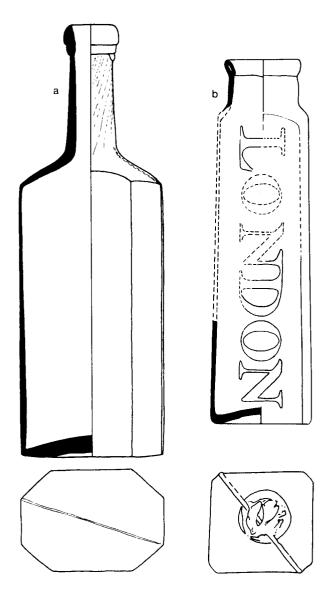
Figure 7. Two examples of two-piece moulded bottles. (a) A probable sauce bottle. (b) A London mustard bottle. In both cases the mould seam crosses the base and is concealed in the corners of the flat-sided body.
