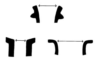
Figure 84. Bore diameter.
