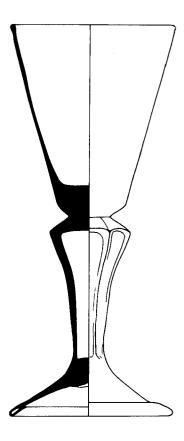
Figure 8. The stem of this drinking glass has been mould blown and attached to a free-formed foot and bowl. The mould seam stops below the bowl and at the foot-stem junction.
