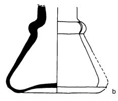
Figure 27. (a) The base of this bottle has been formed by an oval-shaped post and the body shaped in a two-piece mould. (b) An ink bottle manufactured by a two-piece mould and separate cup base mould.
