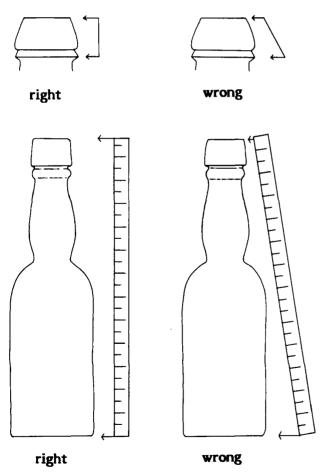
Figure 83. Taking measurements.
