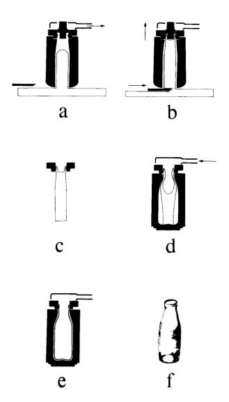
Figure 16. Mechanical forming of glass containers: the Owens suction-and-blow process. (a) The gob is sucked up into the blank mould. (b) The neck of the container is formed and the glass gob sheared off at the base. (c) The blank or parison shape with the ring mould still attached. (d) The blank shape is transferred to a full-sized mould and blowing begins. (e) The container's final shape is blown. (f) A finished bottle.
