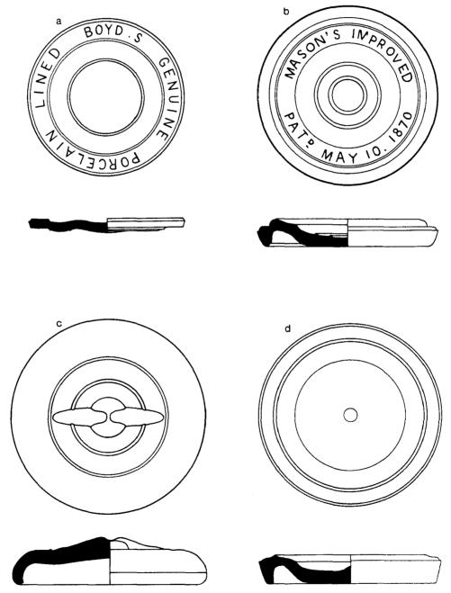
Figure 142. Glass liners. (a) Boyd's Genuine Porcelain Liner in opaque white glass. (b) Mason's improved liner. (c) Liner from a lightning closure showing the moulded centring configuration. (d) Plain glass liner with mamelon.
