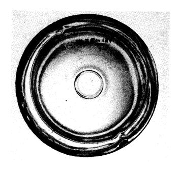
Figure 23. A valve mark on a bottle base. Toulouse (1969: 583) says that this mark is caused by a valve that ejects the parison out of the mould so that it can be transferred to the blow mould for completion.
