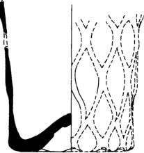
Figure 12. This tumbler has been manufactured by pattern moulding. The diamonds are more concentrated at the bottom of the object and diffused at the top, and the interior and exterior glass surfaces have corresponding contours (cf. contact-moulded examples, Fig. 5).
