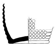
Figure 5. Examples of contact-moulded glassware. Note that the interior and exterior surfaces of the glass are parallel to each other.
