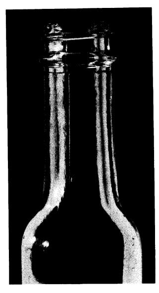
Figure 21. Close-up view of a container finish, showing the large number of seams by the mould parts.
