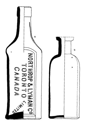
rigure 29. Two bottles blown in vented moulds. (a) Has one vent mark on the shoulder and the bumpy appearance of the letters is accounted for by vent holes in many of the letters. (b) Has two vent marks on the shoulder with two more on the opposite side of the bottle.
