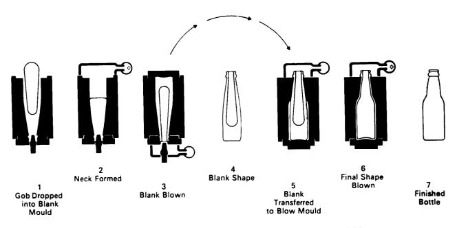
Figure 17. Mechanical forming of glass containers: the blow-and-blow process. (Published with permission of Glass Manufacturers Federation 1973: 25.)
