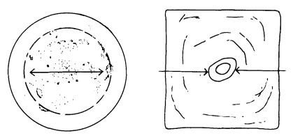
Figure 99. Pontil mark diameter.
