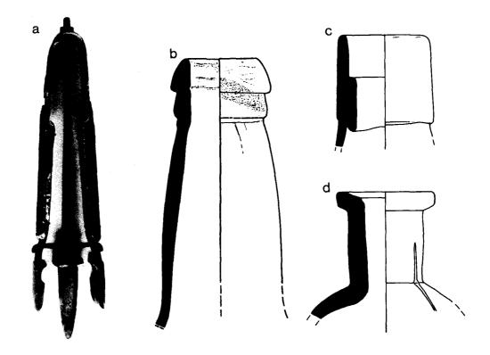
Figure 25. (a) Finishing tool. (b, c, and d) Three examples of finishes formed by finishing tools with different configurations on the plug and jaws of the clamp.
