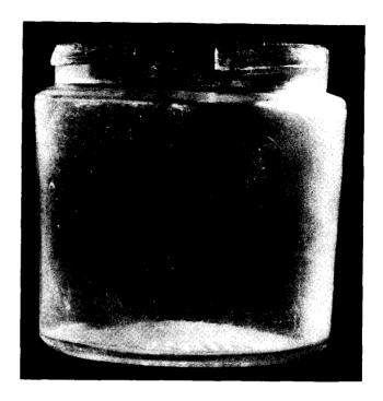
Figure 24. Jar manufactured in a finish-forming mould. Mould seams run the length of the object and the lip has been ground flat.
