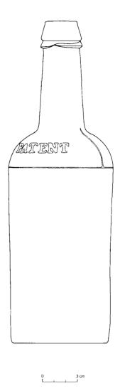
Figure 10. A Ricketts-type moulded liquor bottle, showing the characteristic mould lines on the shoulder.
