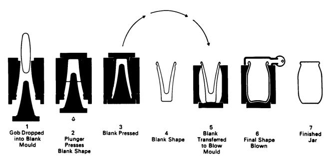
Figure 18. Mechanical forming of glass containers: the press-and-blow process. (Published with permission of Glass Manufacturers Federation 1973: 25.)
