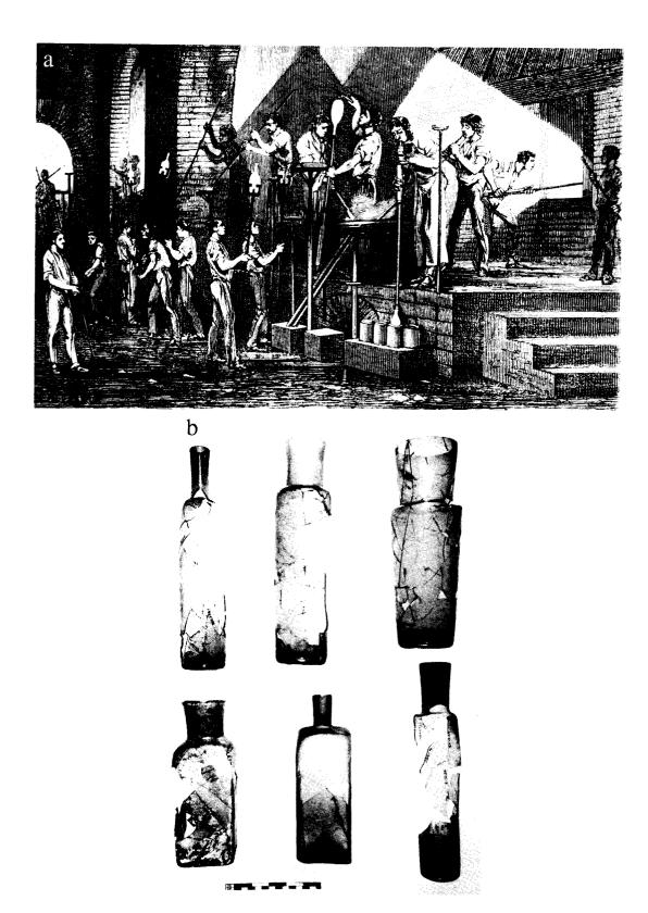
Figure 6. (a) One glassmaker is blowing hot glass into one of a bank of dip moulds (Peligot 1877: Fig. 47). (b) A selection of French blue-green bubbled glass bottles made by the dip-moulded process. These examples show the use of similar body moulds with differing neck styles.
