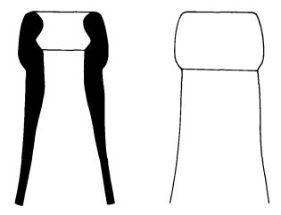
Figure 146. A bottle with a finish for an internal gasket, possibly the Baltimore Loop Seal, patented in the late-19th century by William Painter (Lief 1965: 16-17).
