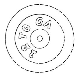
Figure 26. A separate base part which has left its own mould seam on the heel of the bottle. Separate base parts do not always have commercial markings.
