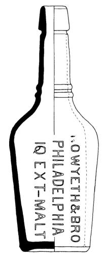
Figure 9. A probable bitters bottle blown in a two-piece mould with a separate base part that leaves a mould seam above the heel of the bottle.
