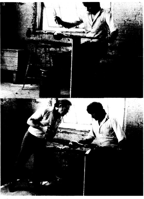
Figure 1a, 1b. Some of the steps involved in the off-hand manufacturing process of a bottle. These photographs were taken at the Chalet Glassworks in Cornwall, Ontario, in May 1972. The glassmakers are using traditional glassworking tools. (a) The neck of the bottle is lengthened by the jacks. (b) Shaping the body with a flat paddle.
