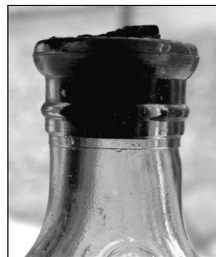
Figure 2-31 – Horizontal machine seam at base of finish
