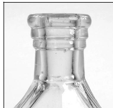
Figure 2-33 – Double reinforced finish or double collar (Lindsey 2010)
