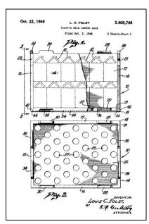
Figure 4-37 – Folst's patent for a plastic case
