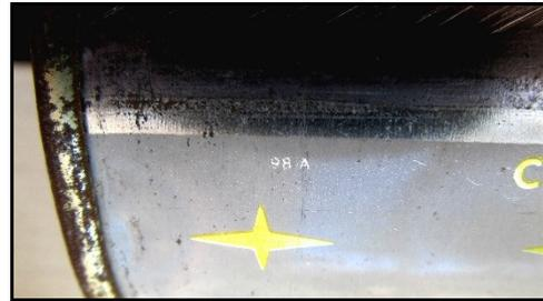
Figure 8b-12 – Tiny 98A beside seam
