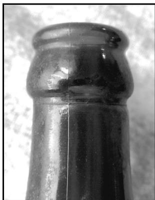
Figure 2-54 – Machine-made finish – note both horizontal and vertical seams
