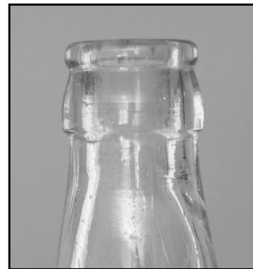
Figure 2-53 – Tooled crown finish – note faint horizontal striations
