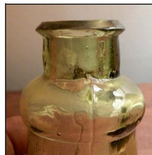
Figure 23 – Side seam on blacking bottle (eBay)
