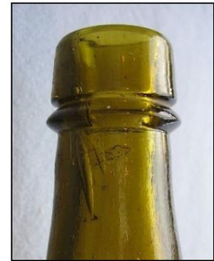
Figure 14 – Two-part finish, sharp lower ring (eBay)
