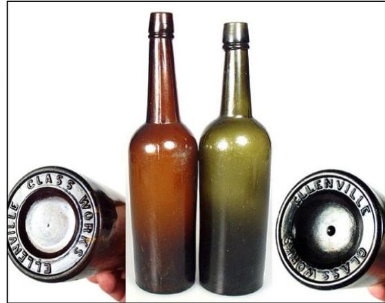
Figure 50 – Indented base – Ellenville Glass Works (on left – concave base on right) (Glassworks Auctions)
