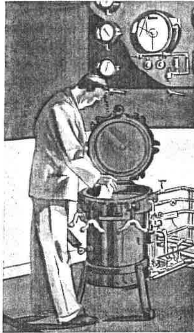
This miniature retort affords the same opportunity for sterilization under pressure as is had by the larger equipment found in canneries. Automatic pressure and temperature controls are combined with it.
