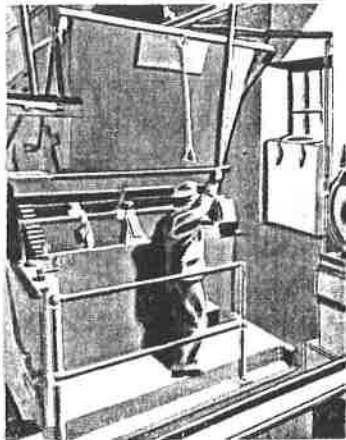
The slightest variation in glass batch may cause endless grief and trouble for the furnace man. Extreme care is used in weighing raw materials.
