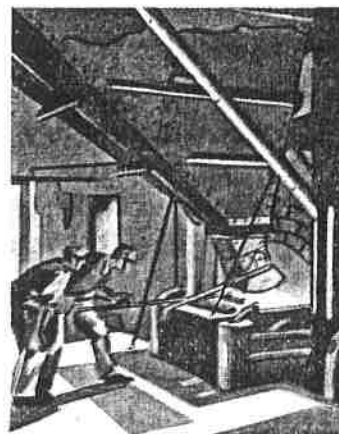
At regular intervals new batch is fed into the furnace mouth, familiarly known as the "Dog House". It's a hot job requiring no little intelligence and skill.
