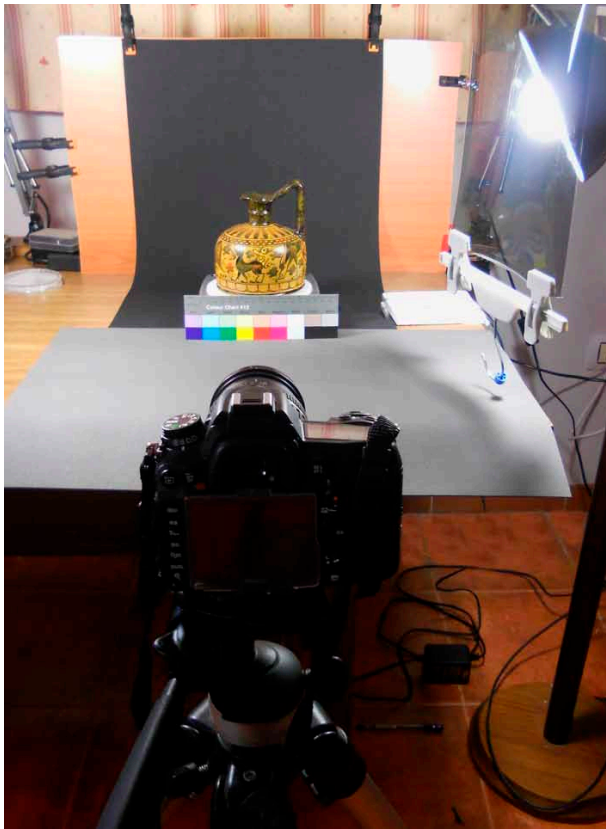
Figure 1. The basic arrangement for the rollout photography. This replica of Greek Corinthian pottery is on a motorized turntable to shoot a control photograph with a color template card. The light on the right has a linear polarized sheet covering it. (Photo by author, 2011.)
