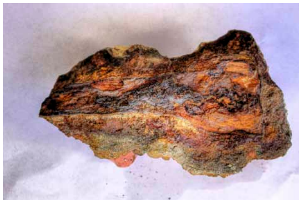
Figure 3. The resulting HDR image clearly defines the outline of the remaining iron running through the center of the concretion. The large areas of corrosion around the head of the nail are better defined in this image. Generally, iron that has been bent or hammered during the manufacturing process is more susceptible to corrosion. (Photograph by author, 2010.)
