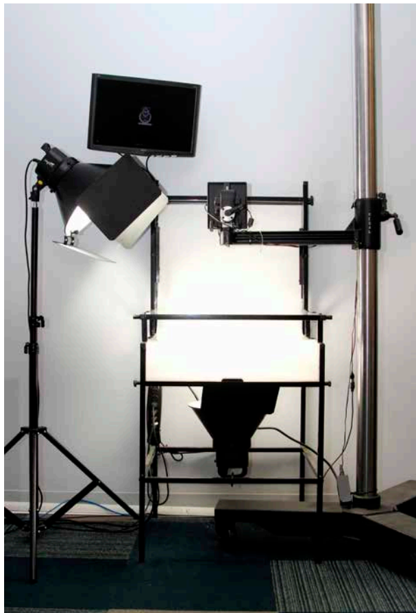
Figure 3. A plexiglass shooting table with a light source beneath it creates the effect of a seamless white background, while the weighted mono stand allows for precise composition and focus. (Photo by author, 2014.)
