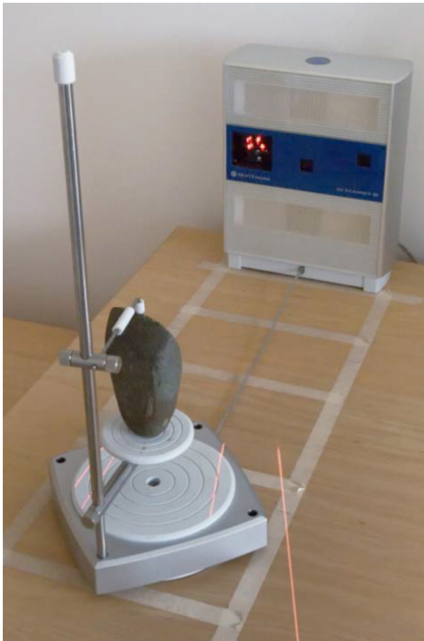
Figure 2. NextEngine Desktop 3D Scanner working in wide mode with the adze on the turntable. (Photo by Ángel M. Felicísimo, 2013.)
