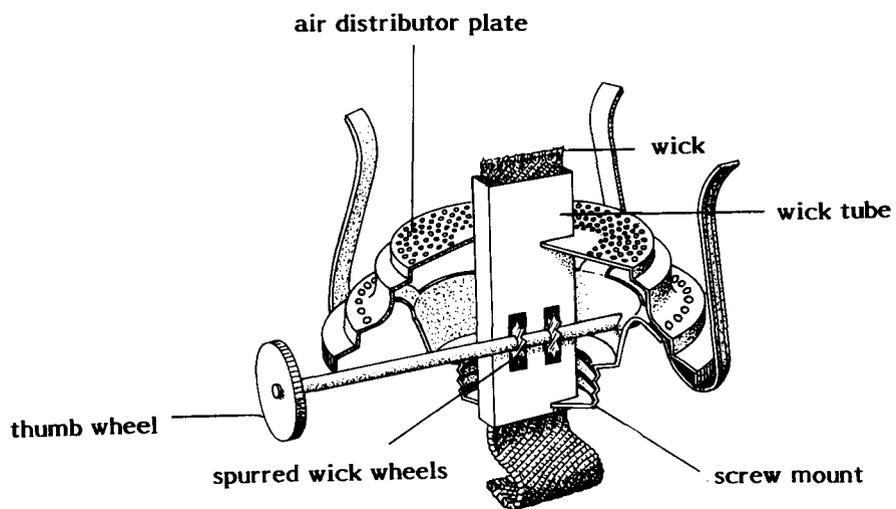
**Figure 46.** Nomenclature of vertical wick lamp burner. (Drawing by D. Kappler.)
