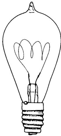
**Figure 73.** Miniature incandescent lamp (1U2A1-318). Height: 7.2 cm. The single multiple-looped filament is of unidentified composition. There is a pumping opening at the top, the bulb is clear, and the screw-type base is copper. Approximate date: very late 19th century or very early 20th century. Small lamps of this type were often made to be mounted in series (garlands or borders) for decoration or advertising.
