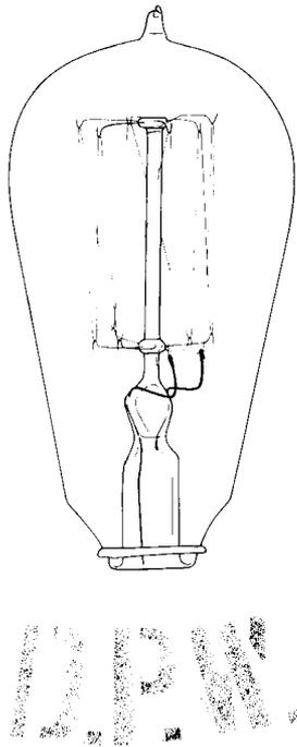
**Figure 76.** Incandescent lamp and customer mark (1U5A1-21). Height: 12.0 cm (without base). The single wire filament forms a cage, fastened by numerous metallic supports to a central glass tube extending the bulb. Composition: probably tungsten or tantalum. Clear bulb. Approximate date: first quarter of the 20th century. The bulb shows, engraved in acid, the initials DPW, likely those of the client, the Department of Public Works. General use impossible to determine. (Drawing by D. Kappler.)
