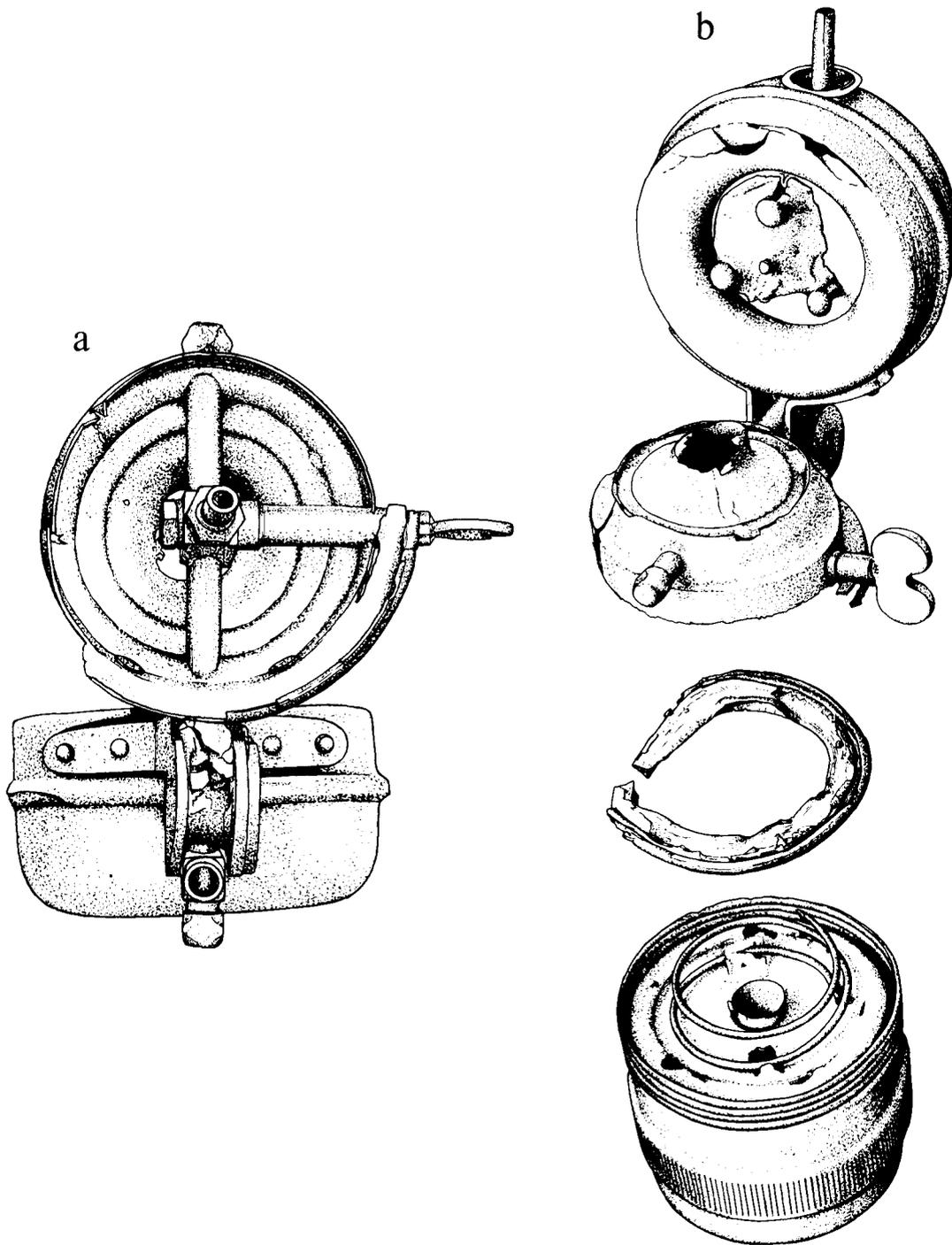
Figure 68. Acetylene lamp for a bicycle. (a) View of the bottom of the cover. (b) Blown-up view. (Drawings by D. Kappler.)
