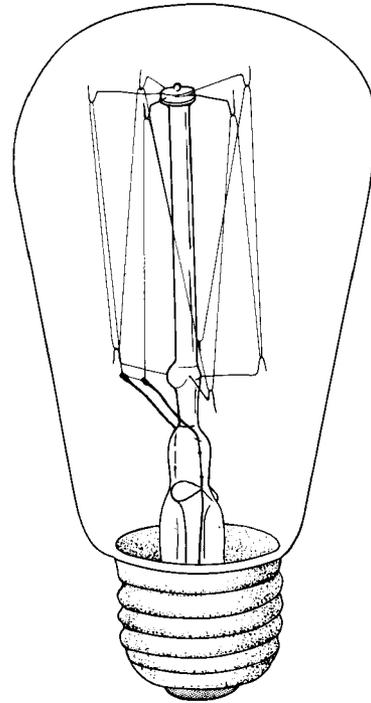
**Figure 77.** Incandescent lamp (1U2A1-298). Height: 11 cm. Single wire filament forming a cage, but more open than that of the preceding lamp. It is fastened in the same way. Clear bulb. Copper screw-type base. Approximate date: first quarter of the 20th century. Use is mainly domestic, but perhaps also commercial. (Drawing by D. Kappler.)
