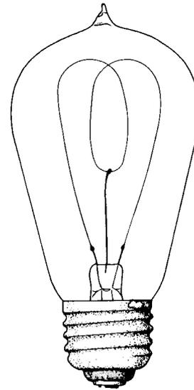
**Figure 72.** Incandescent lamp with its factory mark (1U2A1-82). Height: 11.5 cm. There is a single double-looped filament of unidentified composition. Note the three wire supports directly attached to the bulb. There is a pumping opening at the top, the bulb is clear, and the screw-type base is copper. Manufacturer: Condor, Netherlands. Approximate date: very early 20th century. General usage lamp impossible to specify.
