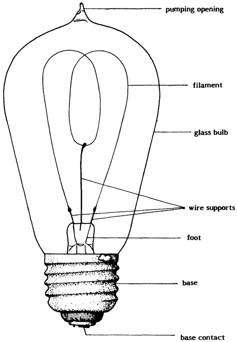
Figure 69. Incandescent lamp and its parts. (Drawing by D. Kappler.)
