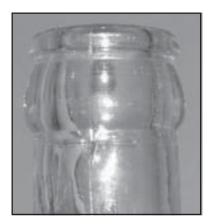
Figure 2: Root Semiautomatic Bottle Finish
