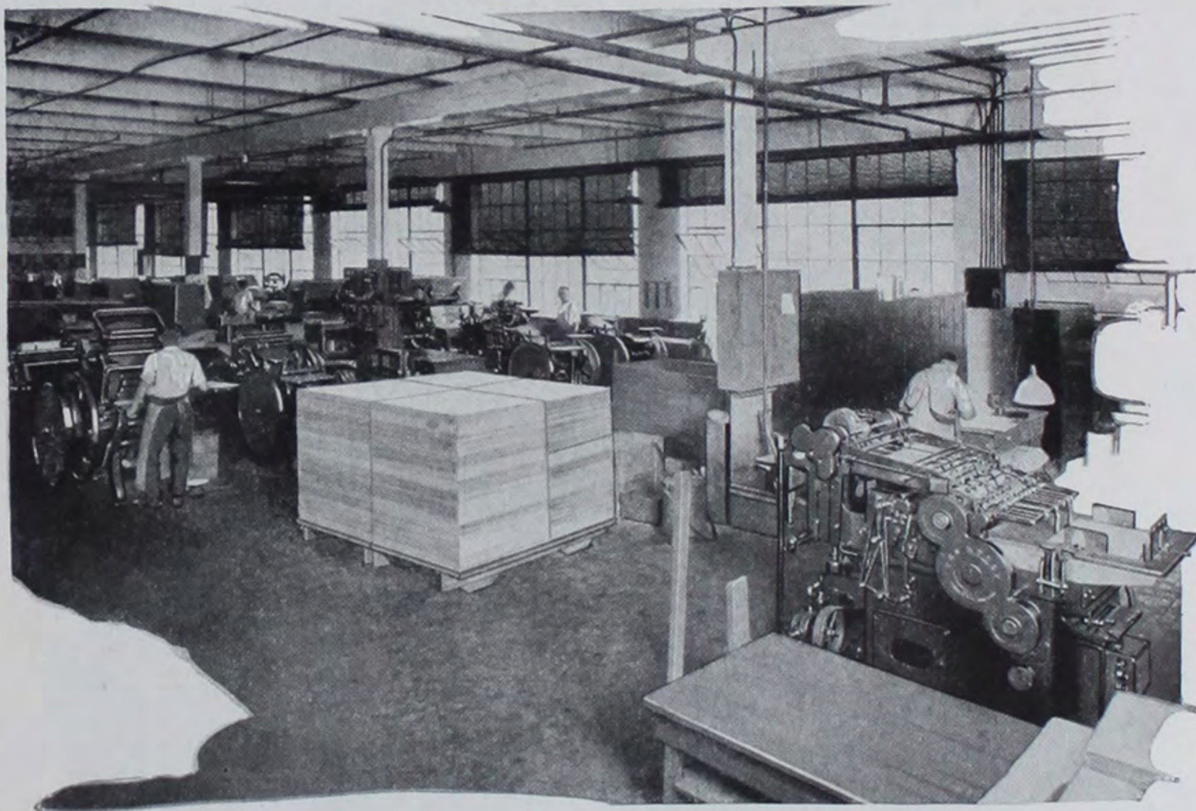
THIS is a corner of the small press division which includes a number of automatic and hand-fed presses, where small orders of labels and cartons are printed before they go to the cutting presses.
