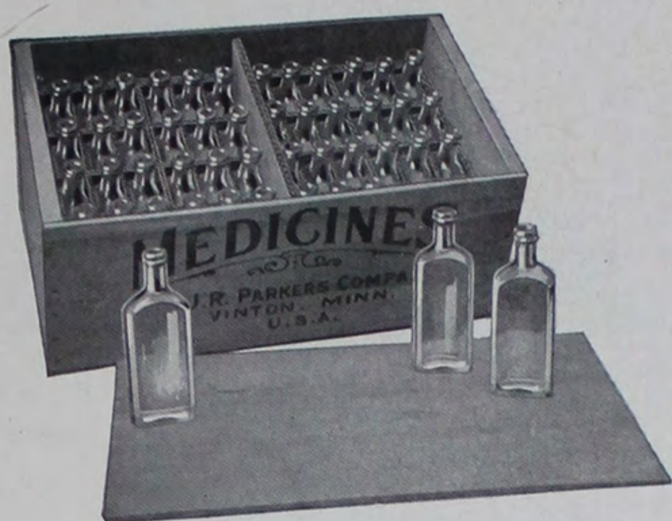
One-tier box, shoulder height partition packing
