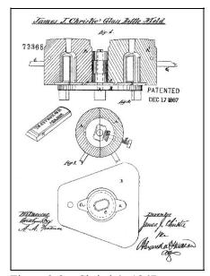
Figure 2-8 – Christie's 1867 patent for plate molds
