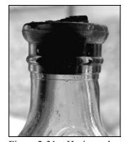
Figure 2-31 – Horizontal machine seam at base of finish
