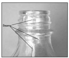
Figure 2-30 – Machine side seam at finish
