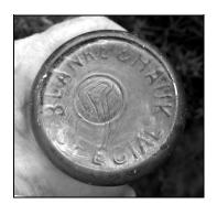
Figure 6-26 – Ejection scar on Type 3 bottle
