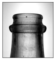
Figure 5-26 – Later Dacro finish with bumper roll
