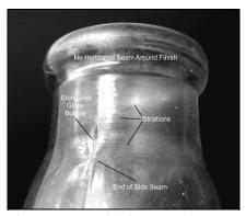
Figure 2-29 – Finish created by mouth-blown process
