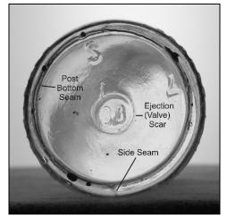
Figure 2-34 – Base created by the pressand-blow machine process
