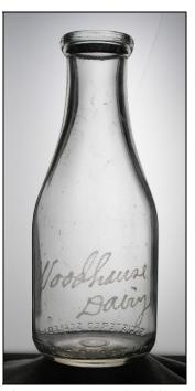
Figure 2-43 – Hand etching
