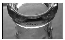
Figure 2-33 – Washboards on neck created by the press-and-blow machine process
