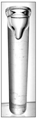
Figure 2-31 – Parison created by the press-and-blow machine process (Courtesy of Jay Hawkins)
