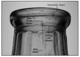
Figure 2-35 – Finish created by the Owens blow-and-blow machine process
