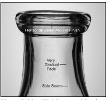
Figure 2-32 – Finish created by the press-and-blow machine process
