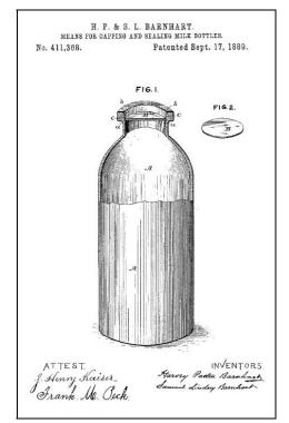
Figure 3-3 – Banhart brothers patent for the Common Sense Milk Bottle
