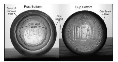
Figure 2-30 – Base created by mouth-blown process
