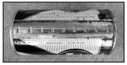
Figure 5b-28 – Side seam of final Liston Azul can
