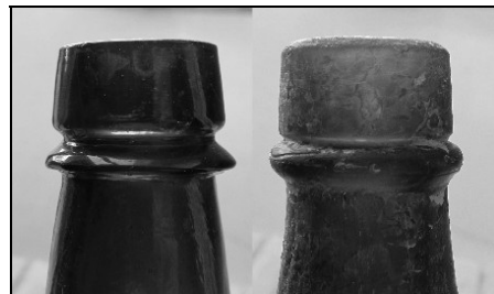
Figure 23 – Export beer bottle finishes with rounded and sharp lower rings
