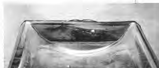
Figure 11 – Fin at the intersection of the base and heel
